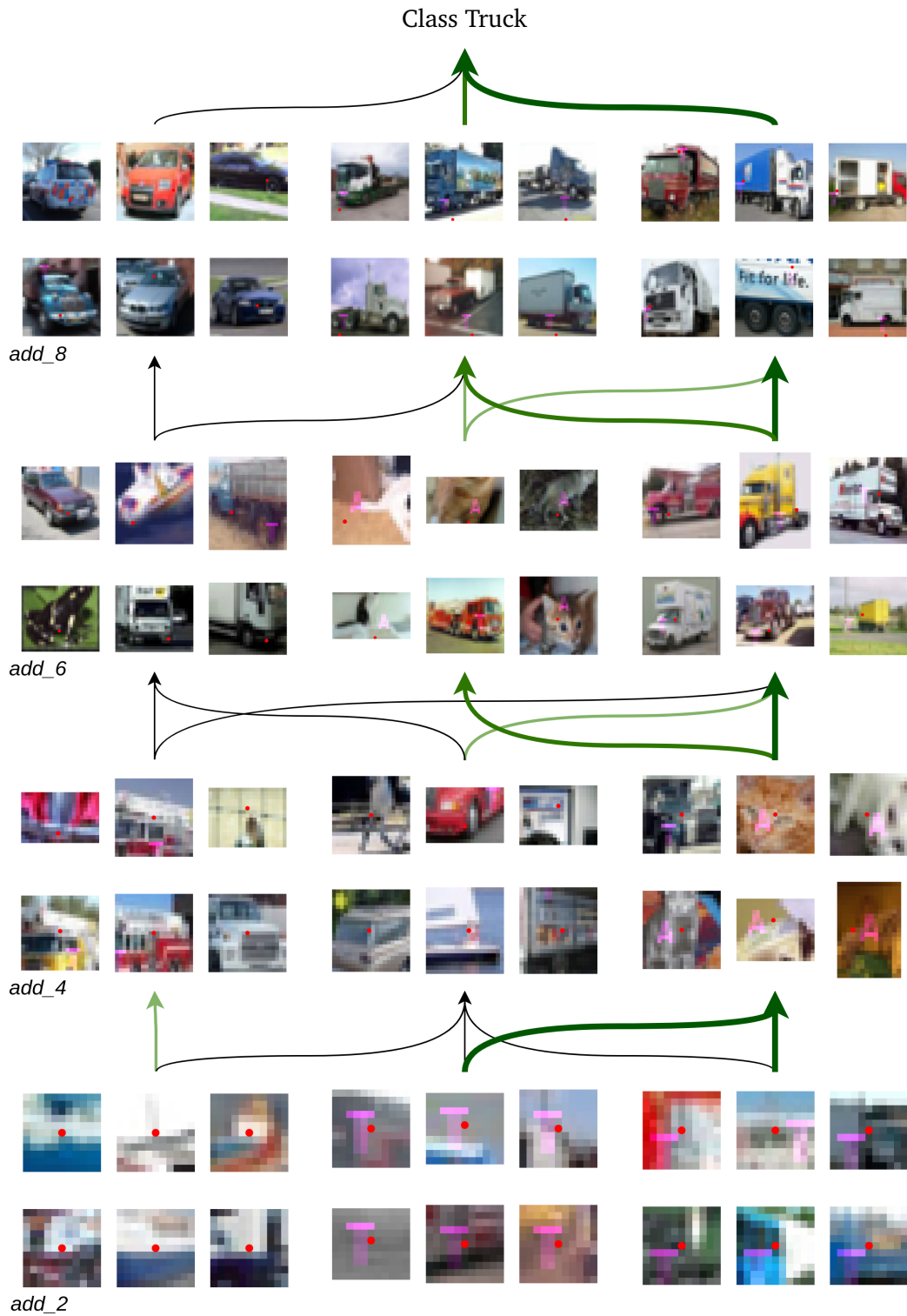
Figure. 2.13: Corrupted data debugging with SIGN. Class inference graph of "truck" class from ResNet20, trained on biased CIFAR10. The data was corrupted by inducing 2 classes with transparent watermarks ( \alpha = 0.5 ) at random places. The above graph shows the "truck" class inference graph in an experiment where classes "truck" and "cat" were corrupted with purple letters "T" and "A" respectively. It is recommended to zoom in for better inspection.
