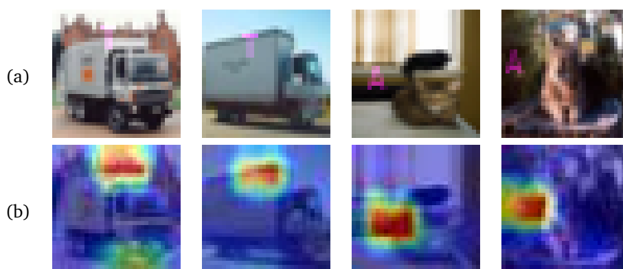
Figure. 2.14: Attention maps demonstration on biased data. (a) Examples of CIFAR10 images corrupted with transparent watermarks along with their (b) corresponding Grad-CAM [9] heatmaps.
